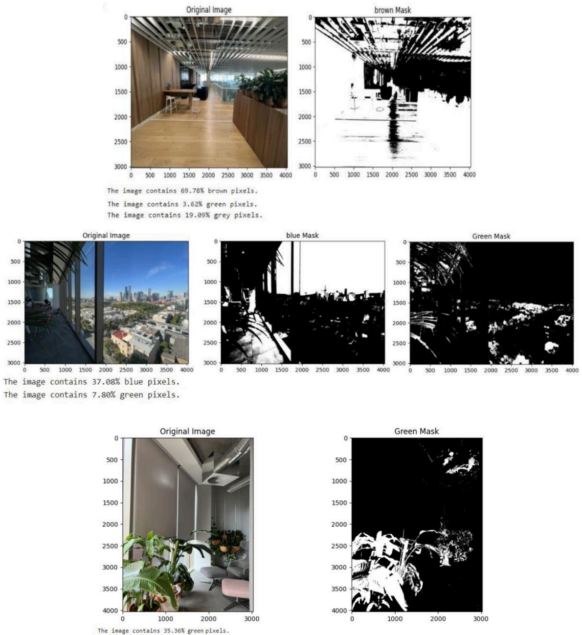
Figure 2. Examples of BD elements analysis of the case study. Brown mask: natural material, green mask: greenery, grey mask: natural colour, blue mask: view to outdoor.
